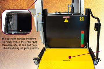
Patented Auto-Index Relief Grinding System allows for both automatic spin and relief grinding with one easy setup. The hands-free operation during the relief grind allows the operator to perform other tasks while the machine does the work.
